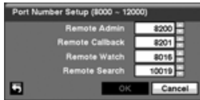
Figure 3-26 Port Numbers Setup Screen
